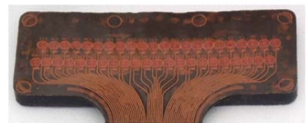
Figure 2 Detail of the PCB flexible ECA probe from Eddyfi (3)
